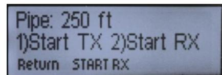
Do not press the CENTER button ("START RX") until the transmitting unit (TX) has started (Step 5). Signal to the operator with the transmitting unit that you are ready for them to start the transmitter.
