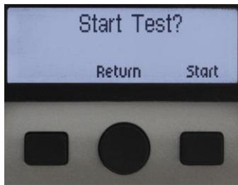
Push the RIGHT button ("START") to begin the test. Once the Transmitter has started (you will hear a series of tones), signal to the operator with the receiving unit to begin listening with the RX unit).
