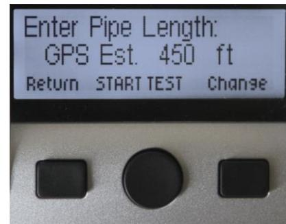
If you agree with the GPS Estimated Pipe Length, then push the CENTER button ("START TEST") to continue. (If you want to adjust the pipe length, push the RIGHT button ("CHANGE") to cycle through various pipe lengths, then push the CENTER button).
