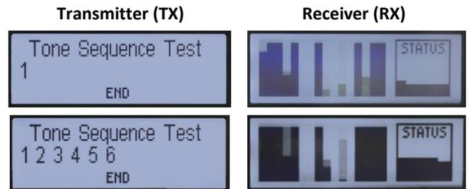
The transmitter will go through a series of tones 6 to 12 times. You can stop this at any time by holding the CENTER ("END") button. Once the test is completed, the RX unit will show some feedback regarding the pipe condition ("GOOD", "FAIR", "POOR", "BLOCK", etc.).
