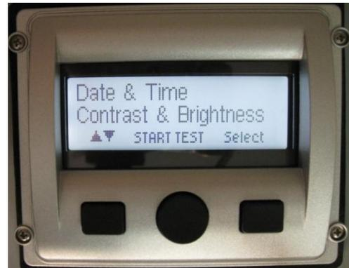
Figure 11 SL-RAT Main Menu - Left Button scrolls the menu; Right Button selects the Top Option.
