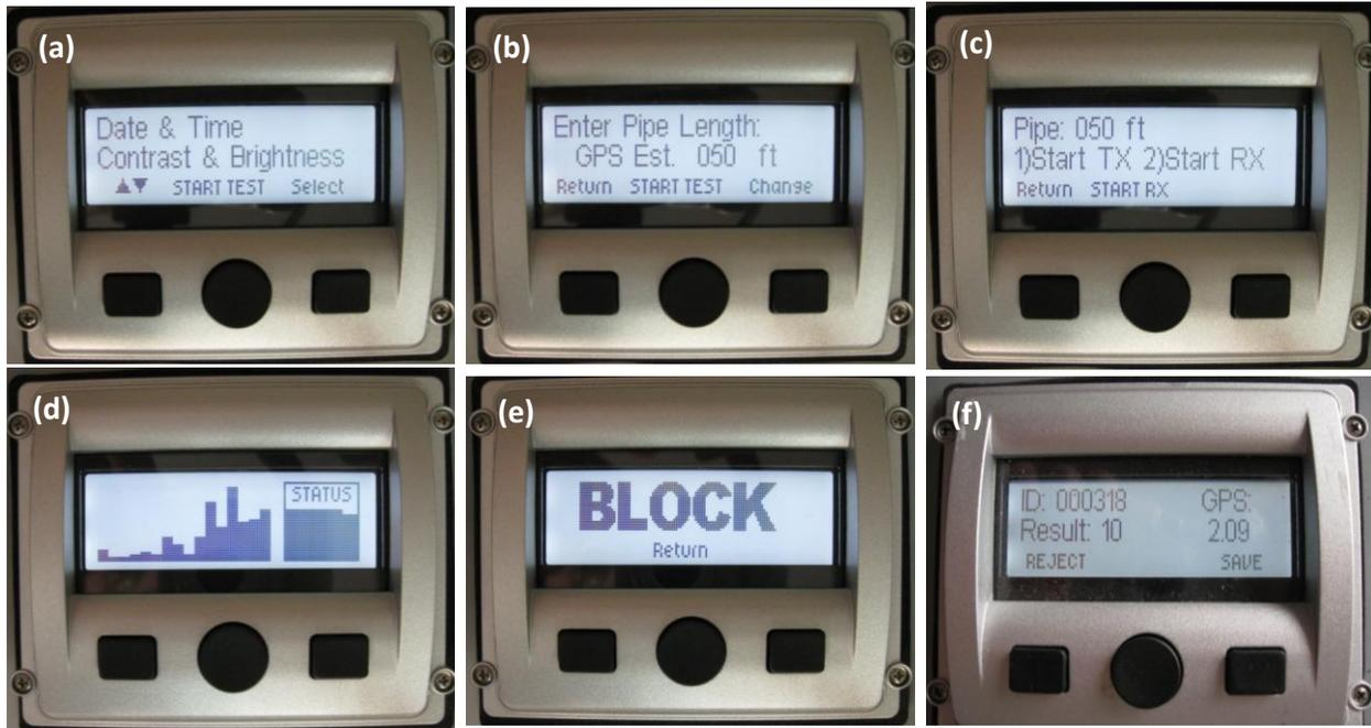
Figure 9 Menu Sequence for RX acoustic measurement operation. (a) Main Menu; (b) Pipe Length Menu; (c) Start Test Instruction Menu; (d) RX Real Time Display; (e) Pipe Segment Assessment; (f) Pipe Segment Evaluation.
