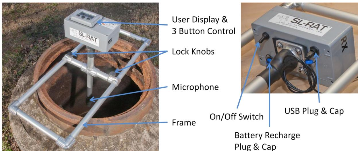
Figure 2 Major sub-components of the SL-RAT™ device's Receiver (RX) Component
