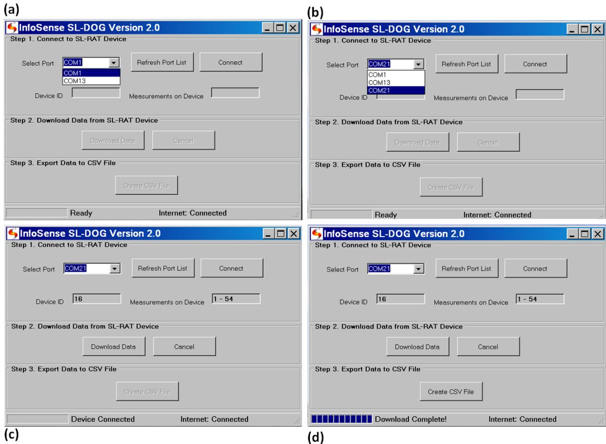
Figure 13 SL-DOG Operation overview. (a) & (b) COM port selection for connecting SL-RAT to SL-DOG; (c) Connection verified and ready to download data; (d) Download complete and ready to create user's measurement data file.
