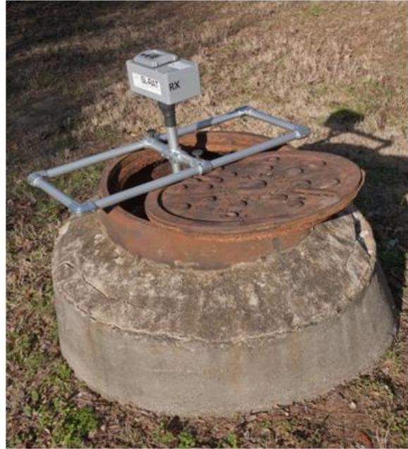
Figure 7 SL-RAT RX deployment with microphone approximately centered and 1' below plane of manhole. Manhole cover only partially removed for the measurement.
