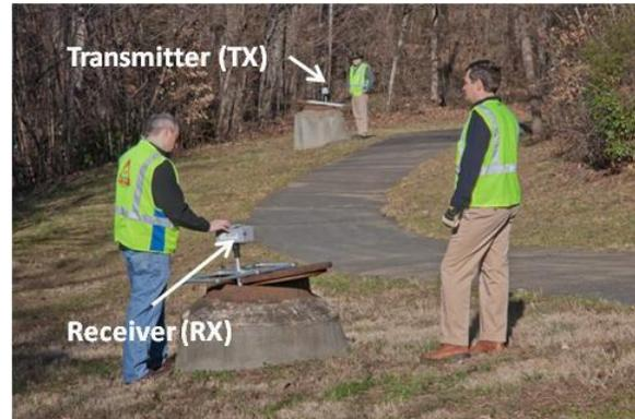
Figure 5 SL-RAT deployment for acoustic measurement of the pipe segment between the two manholes
