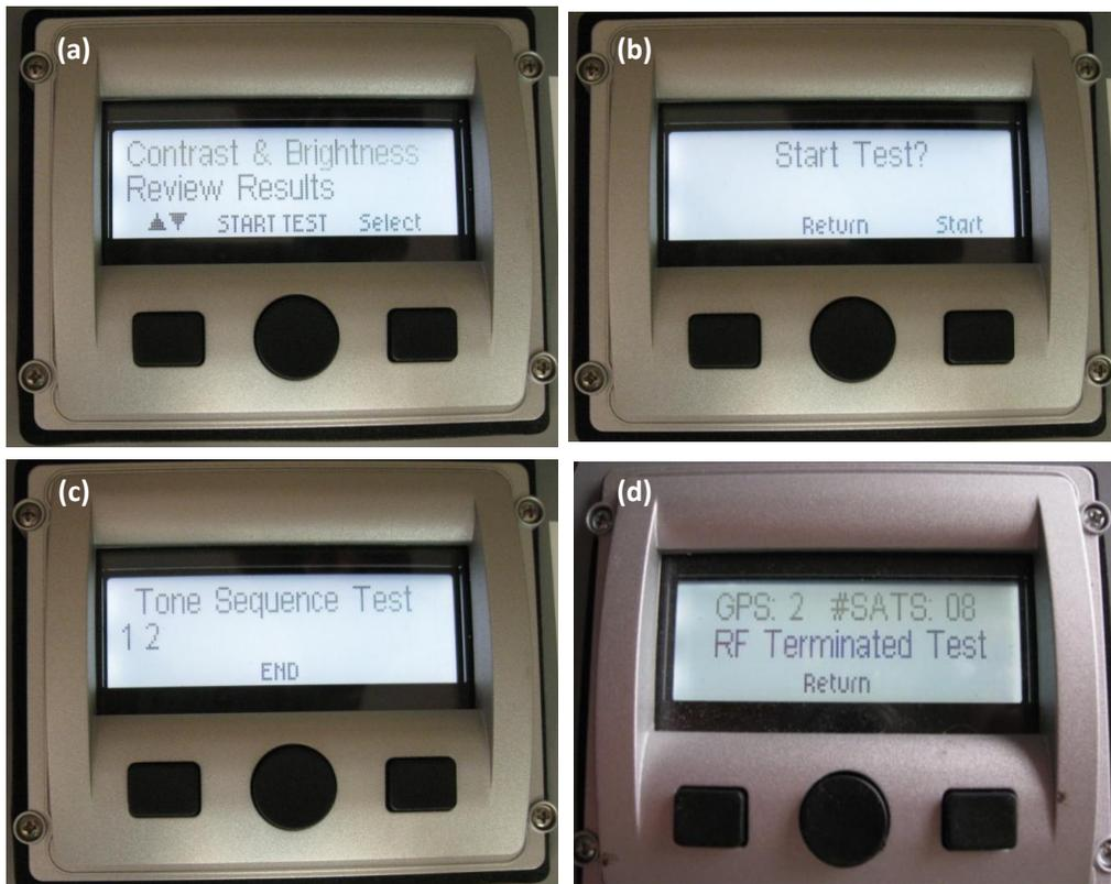
**Figure 8 Menu Sequence for TX acoustic measurement operation. (a) Main Menu - Center Button; (b) Confirm start test - Right Button; (c) TX Measurement Display - count updated after each tone sequence. To end test - Center Button; (d) Return to Main Menu – Center Button.**
