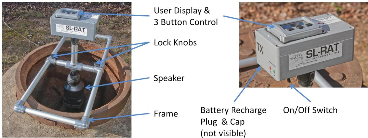
Figure 1 Major sub-components of the SL-RAT™ device's Transmitter (TX) Component
