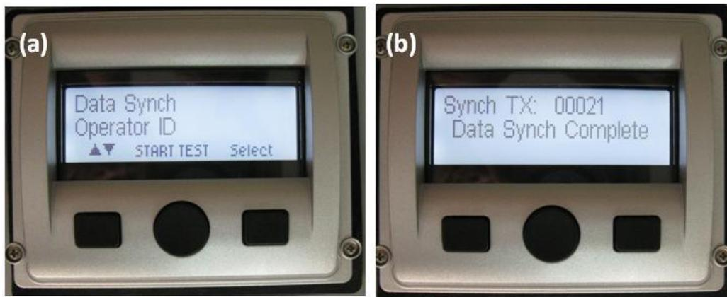
Figure 10 (a) Initiate Data Synchronization from the RX Main Menu when the RX and TX are within 50'. (b) Keep RX and TX within 50' until Data Synchronization is complete.
