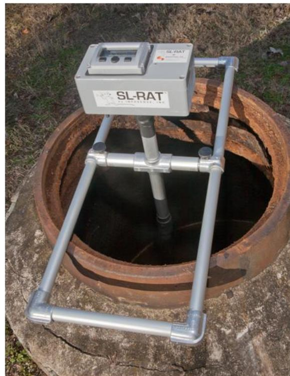
Figure 6 SL-RAT RX deployment with microphone centered and 1' below plane of manhole. Manhole cover removed for the measurement.
